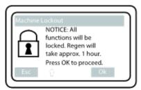
6 Press Ok. If the engine is not already running, the LCD screen will display the message "Start Engine".
